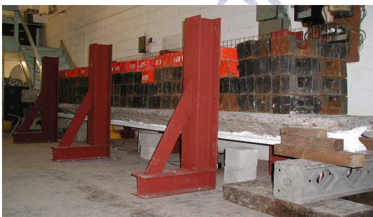
Controlled proof load test of beam in our lab
