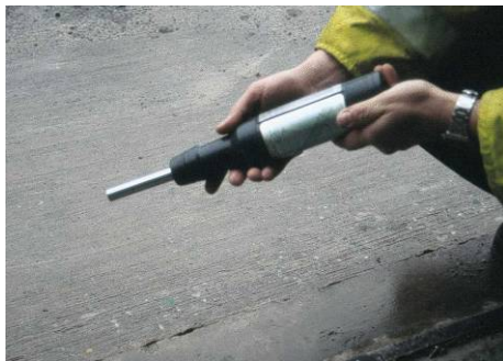
Rebound hammer in use
