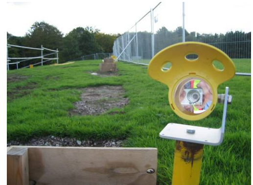
Total station monitoring prism—on the watch for movement
