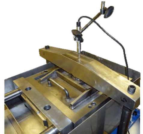
Electronic displacement transducers for measuring vertical displacement.
