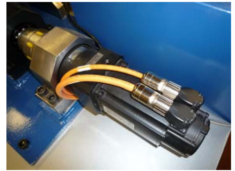
Stepper motor for precision controlled horizontal loading rate.
