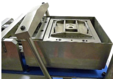
Designed for easy insertion and removal of shear box
