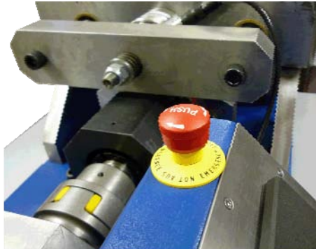
Safety features include overload sensors and emergency stop button
